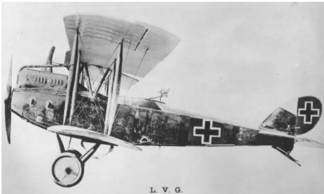
The L.V.G. was an efficient observation aircraft. These German two-seaters, capable of 20,000-foot ceiling by late 1917, often proved to be challenging opponents.
